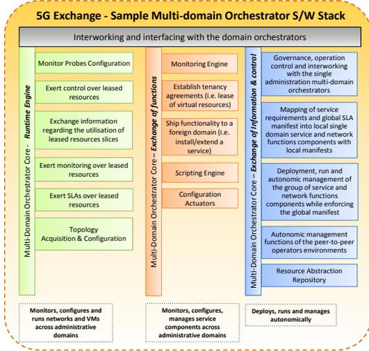
Fig. 2. Sample internal architecture of the Multi-domain orchestrator
